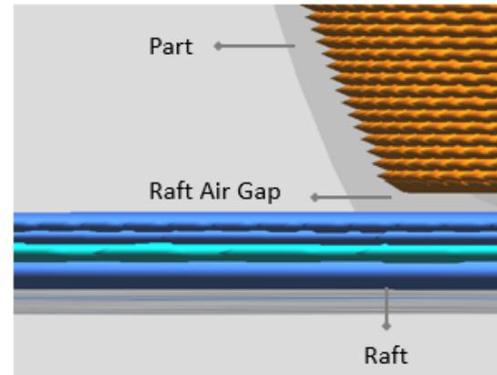
**Note:** If the raft air gap value is set too low, the part will fuse directly to the raft making the removal of the raft very challenging. If the raft air gap value is set too high, the part will not sufficiently adhere to the raft, and the part will warp or not adhere to the build plate at all.
