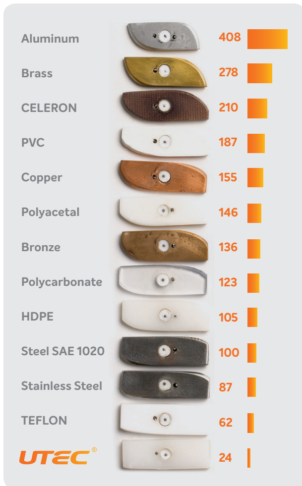
Figure 4 – Relative abrasion wear of UTEC grades and various materials, STEEL SAE 1020 = 100. The pictures show the tested parts. Measured by Braskem internal sand slurry method.
